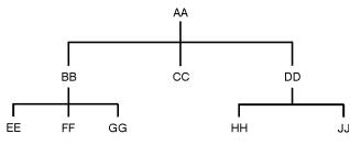
The command closest to the top is the root command, or simply "the root." Notice that you must follow a particular path to reach lower level commands. In the following example, :POWer represents AA, :ALC represents BB, :SOURce represents GG. The complete command path is :POWer:ALC:SOURce? (:AA:BB:GG).
